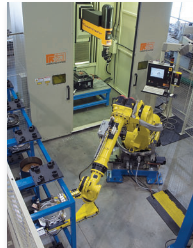
A LASERDYNE system teamed with a robot for part loading and unattended processing. An example of LASERDYNE SYSTEMS commitment to turnkey processing.
