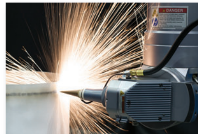
High speed drilling on the fly with a CL50k Nd:YAG laser using LASERDYNE exclusive OFC (Optical Focus Control), BTB (BreakThrough Detection), and CylPerf programming at normal, minor, shallow, and compound angles.
